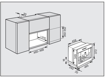
or underneath a wall unit using a special building-under frame **CVUG 50** (available to order)
